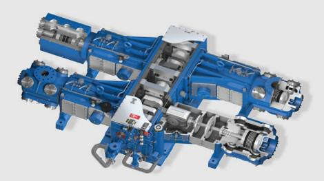
Oil & Gas Systems Limited (OGS) are authorised by Ariel Corporation in the USA, to build compression systems using their range of reciprocating compressors. These are heavy duty, horizontal balanced opposed machines available as 1, 2, 4 or 6 crank throws, in accordance with design codes API 618 (ISO13707) / API 11P (ISO13631).
