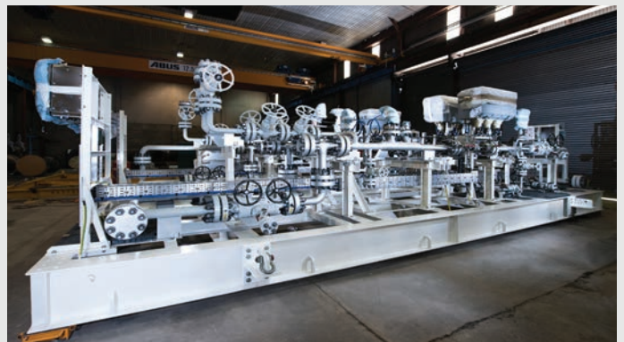
Nexen Petroleum Aoka Mizu Fuel Gas Import Metering System (UK Offshore)
