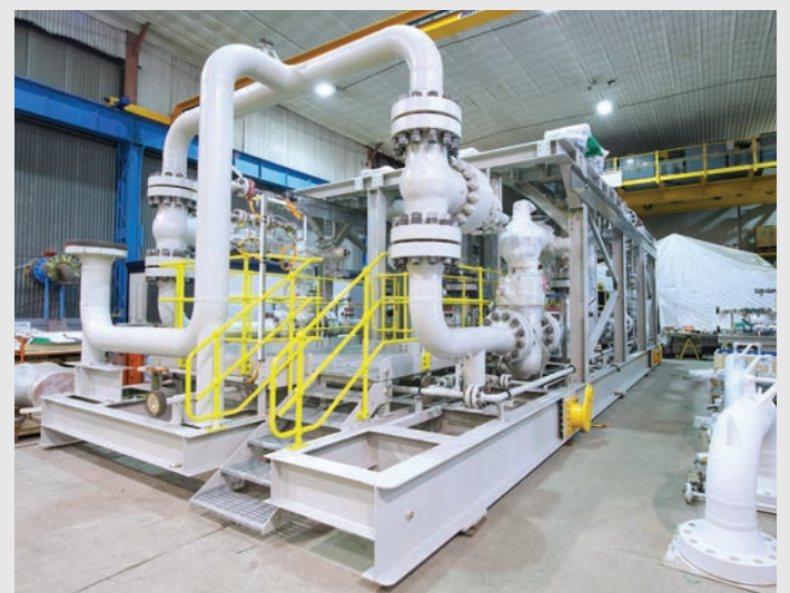
Completed Skid Package
