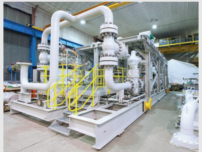
Completed Skid Package
