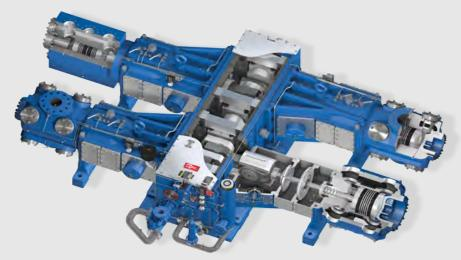
Oil & Gas Systems Limited (OGS) are authorised by Ariel Corporation in the USA, to build compression systems using their range of Reciprocating Compressors. These are heavy duty, horizontal balanced opposed machines available as 1, 2, 4 or 6 crank throws, in accordance with design codes API 618 (ISO13707) / API 11P (ISO13631).
